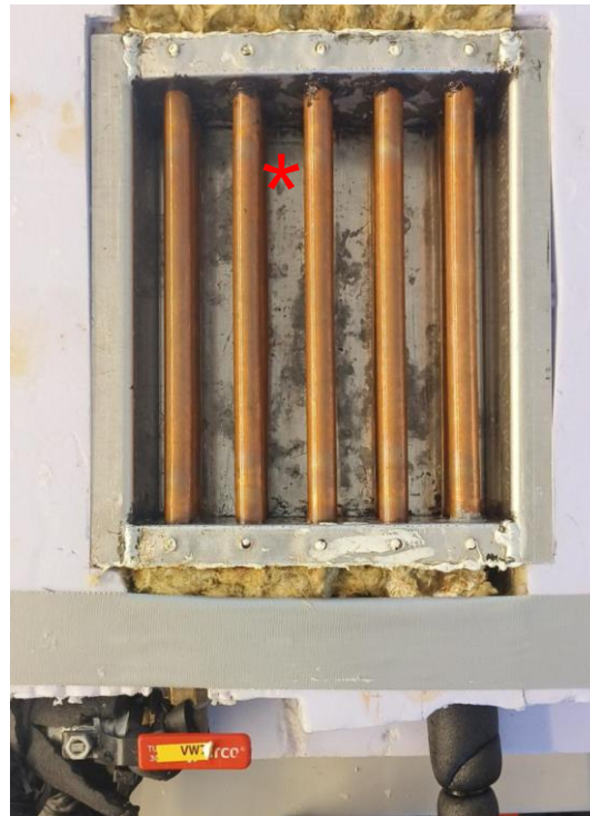
Fig. 6. Picture of the shell-and-tube TES tank (“*” represents the position of the thermocouple) [1].
