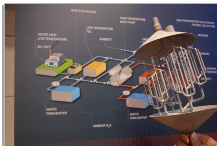
3D model of the Thermal Energy Storage unit – a novel heat exchange system designed to efficiently store and release thermal energy, being developed within the SUSHEAT project by the University of Lleida. (Photo by RTDS Association)
